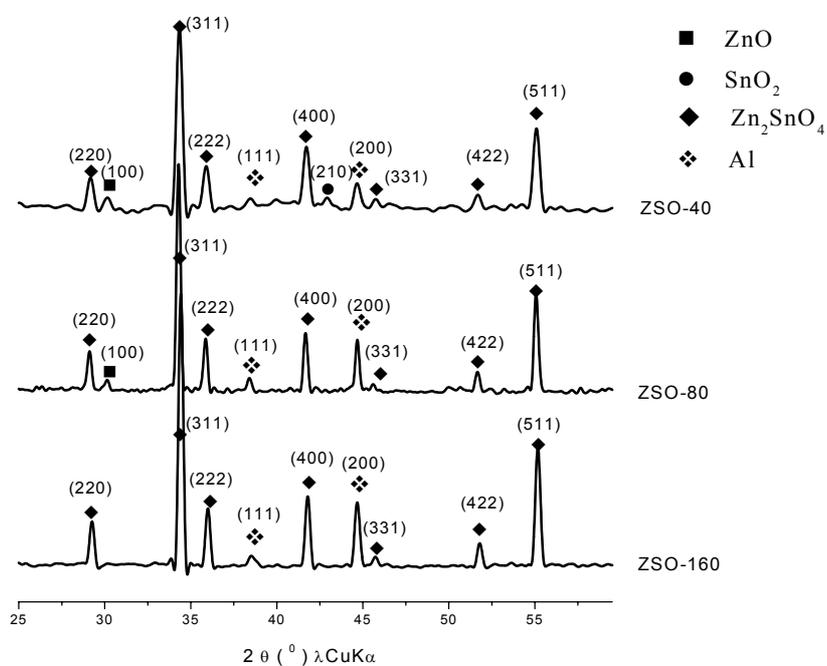
**Fig. 3** XRD patterns of ZSO samples non-isothermally sintered up to 1200°C with a heating rate of 5°C/min.
