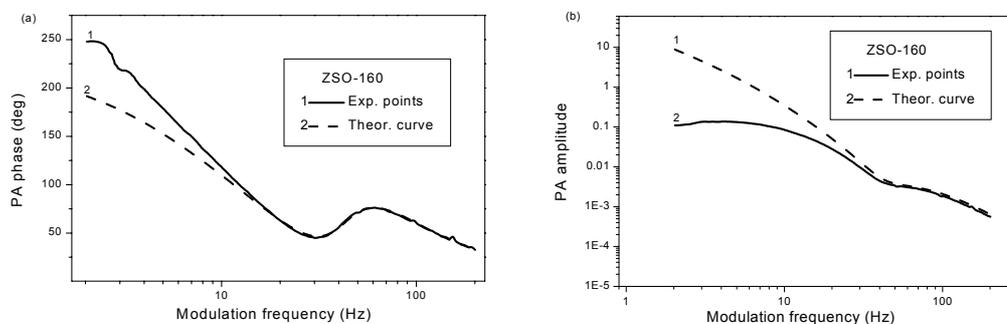
**Fig. 8** (a) Phase photoacoustic spectra for ZSO-160 sample, (b) Amplitude photoacoustic spectra for ZSO-160 sample.
