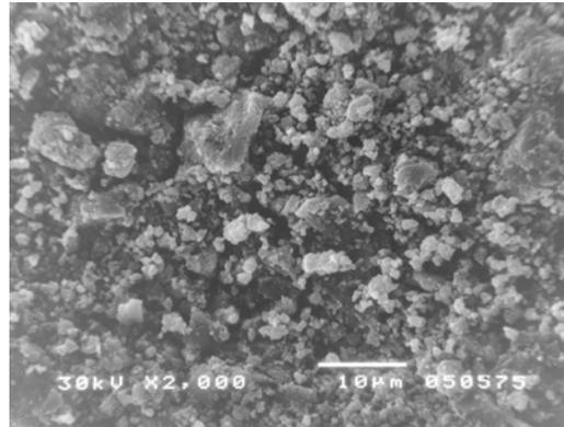
**Fig. 5** SEM fractured surface of the ZSO-80 sample sintered at 1200°C
