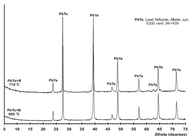
**Fig. 1** X-ray diffractograms of sintered PbTe doped with Boron
