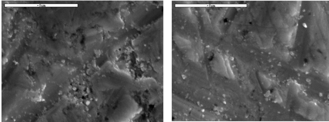
**Fig. 2** Micrographs of PbTe doped with Boron sintered at 600°C (a) and 700°C (b)
