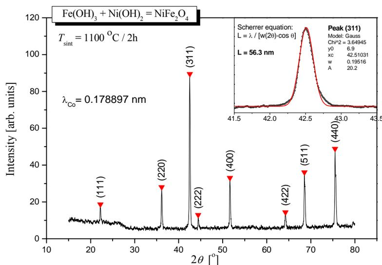
Fig. 1. X-ray diffraction pattern of the  $\text{NiFe}_2\text{O}_4$  sintered at 1100 °C for 2 h.
