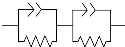
**Fig. 7.** Proposed equivalent circuit model for analysis of the impedance spectroscopy data.
