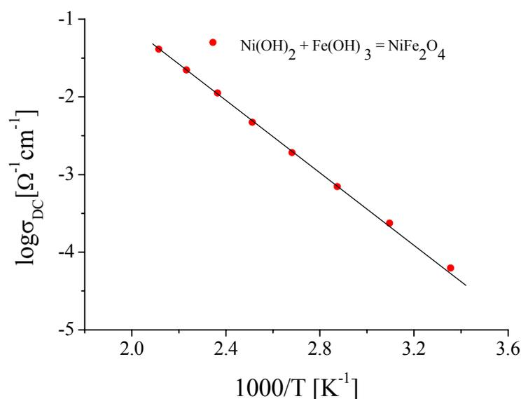
**Fig. 5.** Temperature dependence of DC electrical conductivity of ferrite samples.
