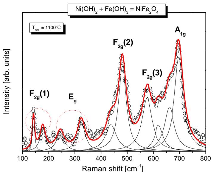
**Fig. 2.** Raman spectra for the sample of the  $\text{NiFe}_2\text{O}_4$  sintered at 1100 °C for 2h.
