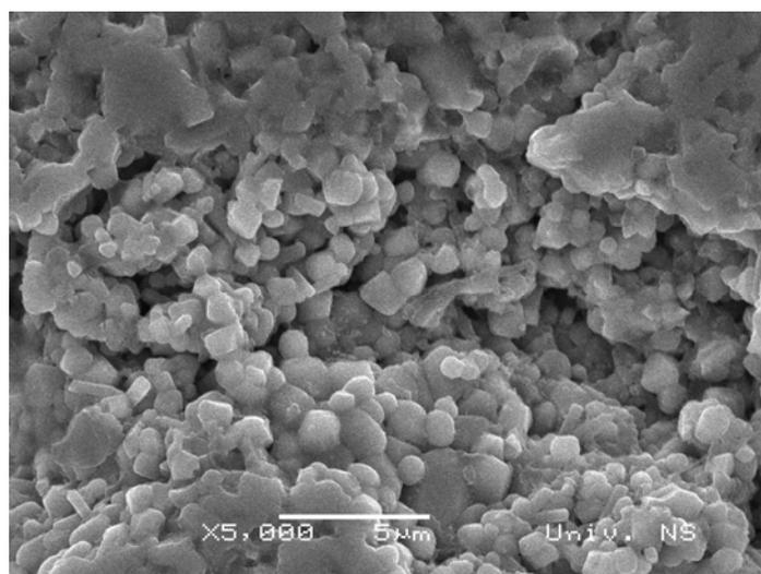
**Fig. 4.** SEM micrograph pattern of the  $\text{NiFe}_2\text{O}_4$  sintered at  $1100\text{ }^\circ\text{C}$  for 2h.
