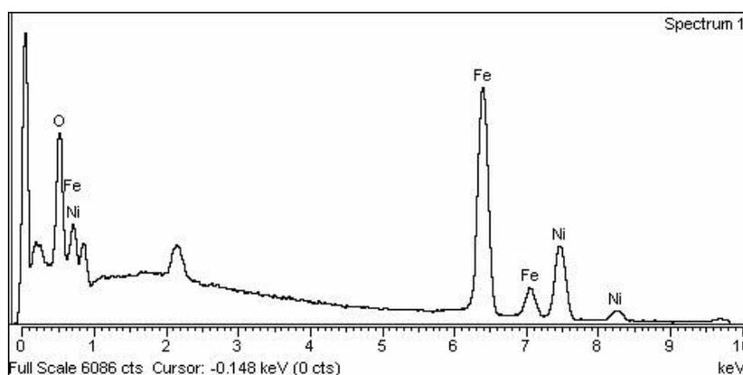
**Fig. 3.** EDS analysis of the  $\text{NiFe}_2\text{O}_4$ .
