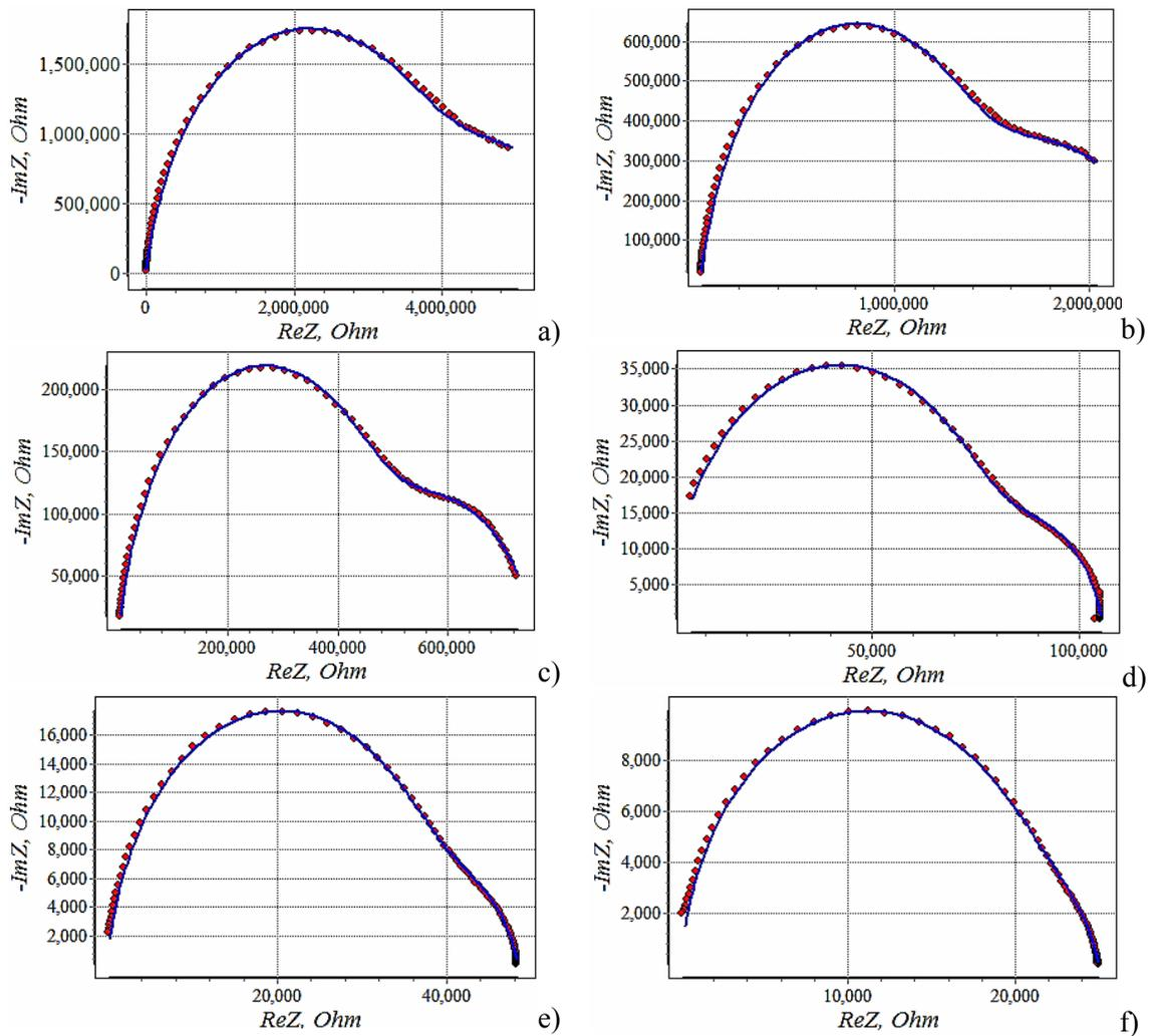
**Fig. 6.** Experimental (red points) and calculated (solid blue line) Cole-Cole plots for  $\text{NiFe}_2\text{O}_4$  ferrite, sintered at  $1100^\circ\text{C}$  and measured at: (a) 298 K, (b) 323 K, (c) 348 K, (d) 398 K, (e) 423 K, (f) 448 K.
