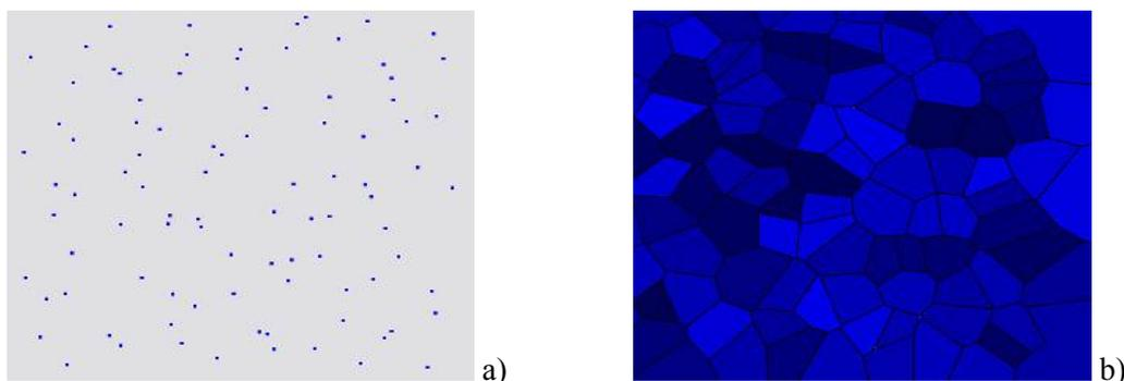
**Fig. 5.** a) Generating set of points which represent the distribution of micro-grains and b) forming set the Voronoi cells.
