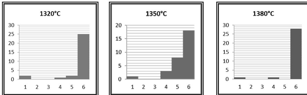
**Fig. 8.** Histograms corresponding to relevant statistical parameters for 0.1 Yb/BaTiO<sub>3</sub> samples, sintered at: a) 1320°C, b) 1350°C and c) 1380°C.
