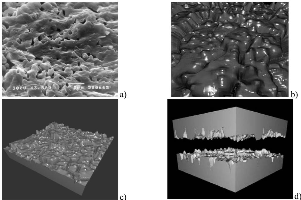
Fig. 7. a) SEM image of Yb doped  $\text{BaTiO}_3$  ceramic, b) micro surface overview profile and c), d) 3D microsurface overview.
