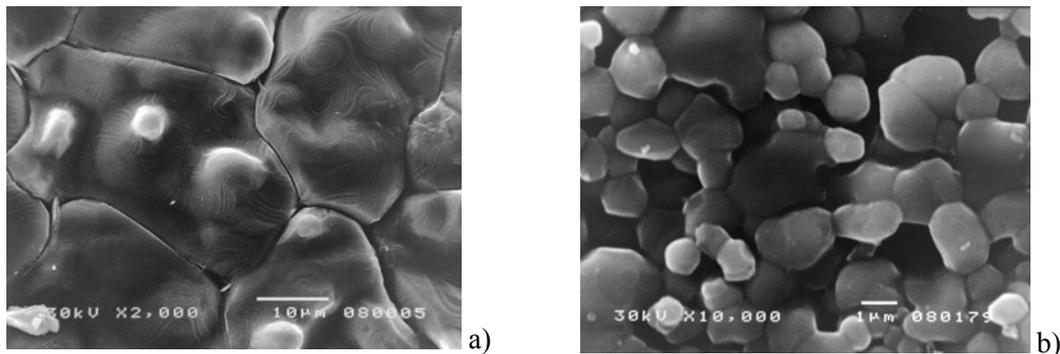
**Fig. 2.** SEM images of Yb doped BaTiO<sub>3</sub> sintered at 1320°C, doped with 0.1wt% and b) 1.0wt% of Yb.
