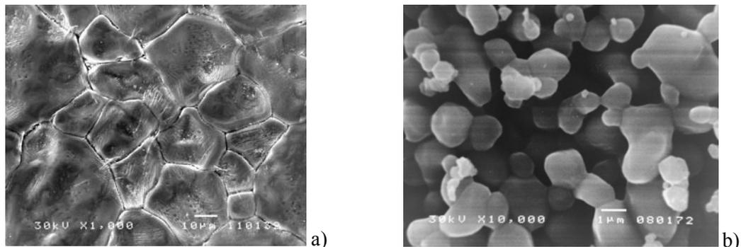
**Fig. 3.** SEM images of Yb doped BaTiO<sub>3</sub> sintered at 1350°C, doped with 0.1wt% and b) 1.0wt% of Yb.
