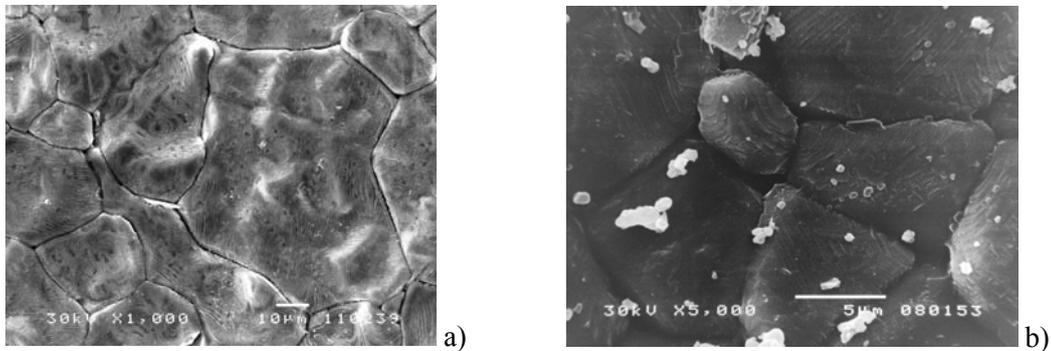
**Fig. 4.** SEM images of Yb doped BaTiO<sub>3</sub> sintered at 1380°C, doped with 0.1wt% and b) 1.0wt% of Yb.
