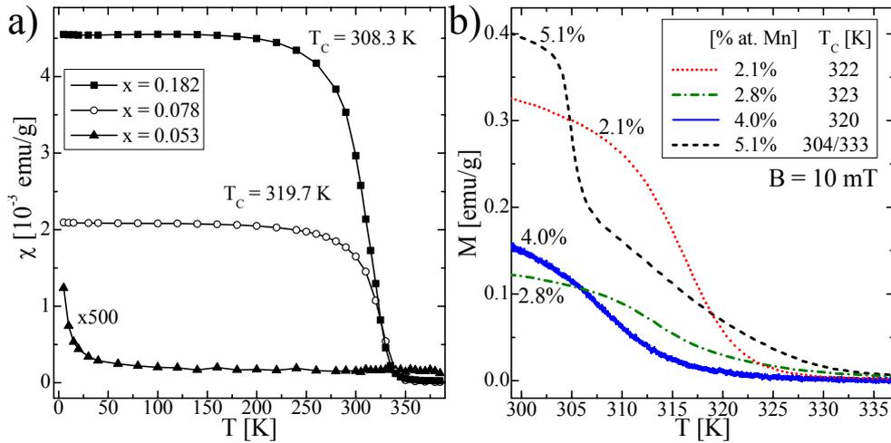
**Fig. 2.** The magnetic properties of Mn-alloyed II-IV-V<sub>2</sub> materials including: (a) the temperature dependence of the magnetic susceptibility for the Zn<sub>1-x</sub>Mn<sub>x</sub>GeAs<sub>2</sub> samples and (b) the temperature dependence of the magnetization for the Zn<sub>1-x</sub>Mn<sub>x</sub>GeAs<sub>2</sub> crystals. Reprinted with permission from L. Kilanski et al., J. Appl. Phys. 108, 073925 (2010). Copyright 2010, AIP Publishing LLC
