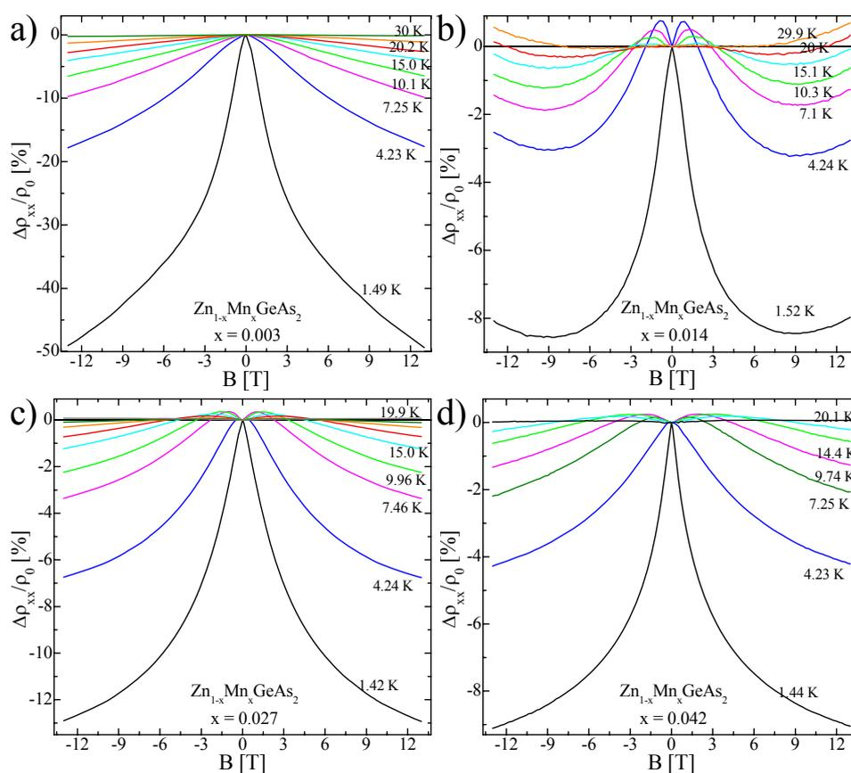
**Fig. 5.** The magnetoresistance curves obtained experimentally at different temperatures for  $\text{Zn}_{1-x}\text{Mn}_x\text{GeAs}_2$  samples with different chemical composition. Reprinted with permission from L. Kilanski et al., J. Appl. Phys. 108, 073925 (2010). Copyright 2010, AIP Publishing LLC. Fig. 1.
